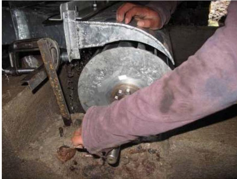
**Figure 30 – The separation between turbine and nozzle**
