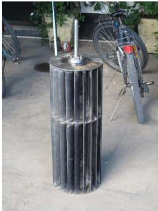
**Figure 8 – The welded turbine runner before galvanising**
