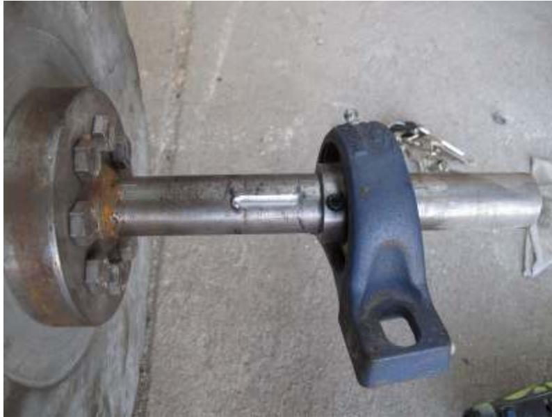
Figure 26 – One of the grooves on the non-driving turbing shaft
