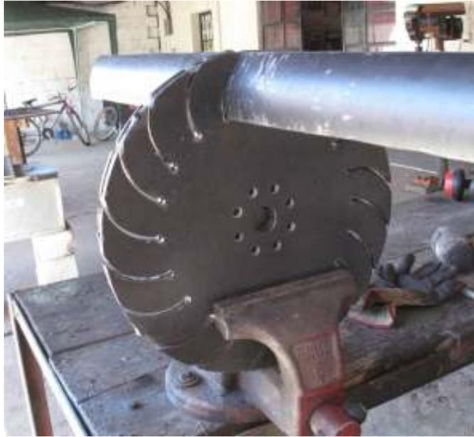
**Figure 7 – End plates with slots cut into them**
