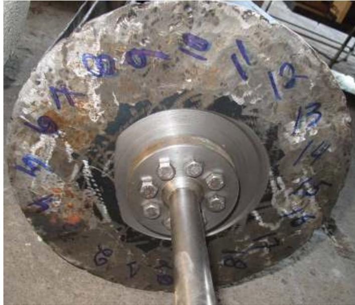
Figure 28 – the shaft hub mounted on the end plate which has been turned in the lathe
