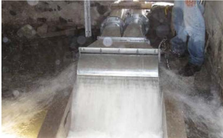
Figure 29 – The turbine operating without side plates at 100% capacity
