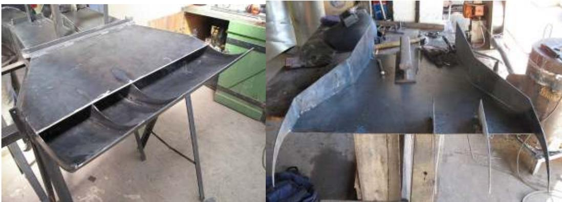
**Figure 21 – The two permanent partitions shown in the finished upside down nozzle (left) and the nozzle before the top plate was welded in place (right)**
