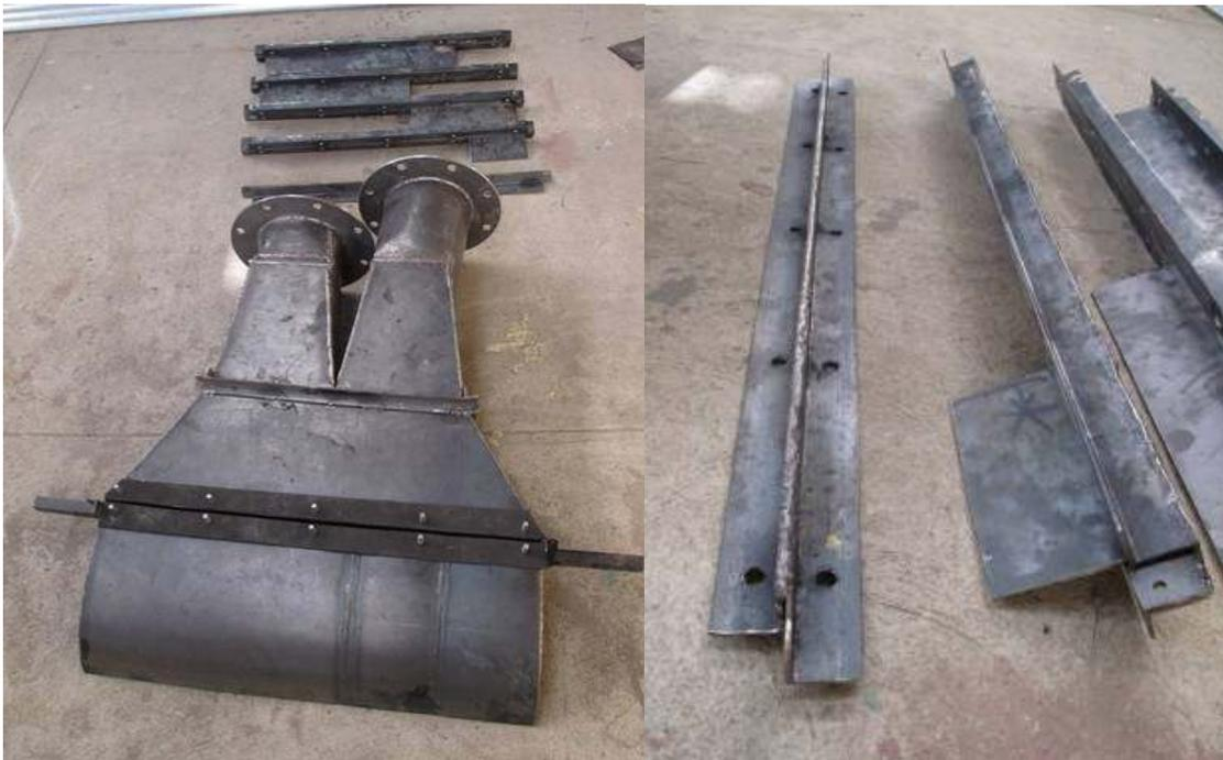
Figure 20 – The nozzle and partition system
